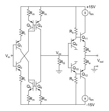
Here, the input transistors  $Q_1$  and  $Q_2$  have a current linearly proportional to  $V_{in}$  by a factor of  $R_i$  (in addition to a constant bias current). We use a pair of current mirrors ( $Q_3$
