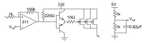
We found that the IRFD9110s had a somewhat higher  $R_{ON}$  than rated. Our power dissipation was actually dominated by static dissipation. Worse, as the switches warmed up,  $R_{ON}$  would increase, and we would have severe thermal runway problems. To combat this problem, we stacked three devices in parallel. This reduced static dissipation to be completely manageable.
