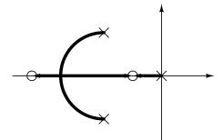
To a first order, we can extend the gain arbitrarily high, until we run into the higher-order poles around the switching frequency, op amp poles, etc.
