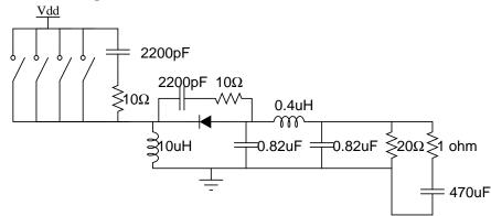
During the design stage, we chose the 1.6pf of output capacitance is chosen to keep switching ripple under 200mV ( $C = I_{out}T_3/V_{ripple}$ ). We found that in practice, although this managed ripple, we still had a large spike due to some switching transient, so we did
