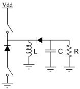
Here, we have three cycles. During  $D_1$ , the inductor is connected to  $V_{DD}$  and charging,  $D_2$  when it is connected to ground, storing charge, and  $D_3$  when it is discharging on the load.
