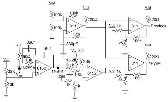
The top left 311 is just a 1MHz Schmidtt trigger oscillator. The bottom left 311 is the compensator. The bottom middle 6152 scales and clips the output of the compensator. The pair of 311s compare the output voltages of the oscillator to the reference voltages to generate the actual PWM and preclock signals.
