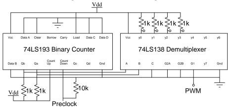
The splitter is just a counter connected to a demultiplexer. The counter selects which switch the input goes to. The demultiplexer actually passes the pulses through to the right switch.
