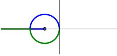
Fig. 4. Shown is the set of pole positions for a pair of poles which give equivalent total time constant. The pair of poles gives the same contribution as a single pole placed at the center of the circle if they are both either on the circle, or if they are both on the real axis with a fixed harmonic mean equal to the position where the circle intersects the real axis.
