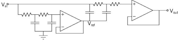
Fig. 5. A cascade of two low-pass filters designed to give 40db/decade passband error roll-off. Here,  $V_{ref}$  follows the signal at low-frequencies.  $V_{out}$  is filtered relative to  $V_{ref}$ , and so has asymptotically better performance in the pass-band.
