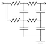
Fig. 8. A passive filter topology that gives 40dB attenuation in the stopband, and 40dB error attenuation in the passband.
