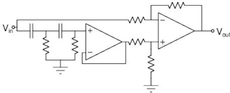
Fig. 7. A lowpass filter with 40dB/dec passband error roll-off, and 20dB/dec stopband roll-off. Passing the signal through multiple such filters would give better stopband roll-off, while maintaining 40dB/dec passband error roll-off. The passband error roll-off is insensitive to component values, but the stopband behavior is limited by the CMRR of the difference amplifier.
